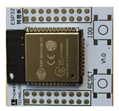
Four contacts have now been soldered, meaning that the ESP32-chip is now fixed and that it would not be able to slip anymore.
