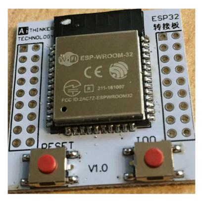
Now that we have soldered all of the SMD contacts, we can solder the pin headers on both sides. To do that, we should take the pin headers and put them on the board:
