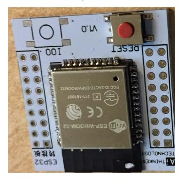
Now you have the possibility again to make a small position adjustment, and again it is recommendable not to heat it up for too long, otherwise, the mechanical button will get damaged.
