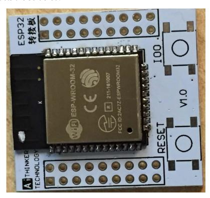
If all contacts of the ESP32 chip are soldered, then we should continue onto soldering the 2 SMD buttons on the board.
